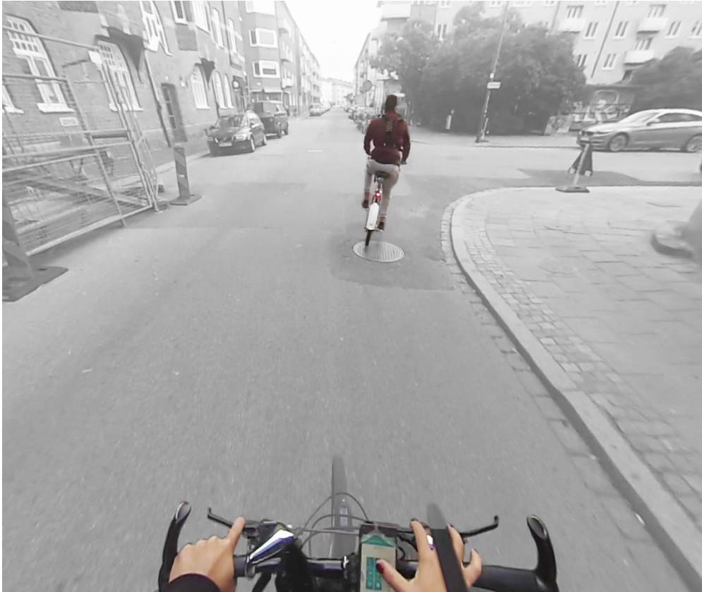
Figure 29: Outdoor test setup. Researcher riding behind the test person, sending navigation commands from a smartphone that is mounted on the handlebar.
