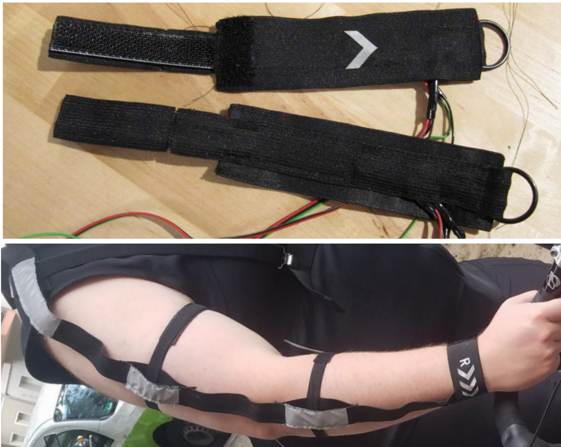
Figure 25: (top) Creation step of the reflective wristbands; (bottom) Attachment of the wristband and cable channel on the arm
