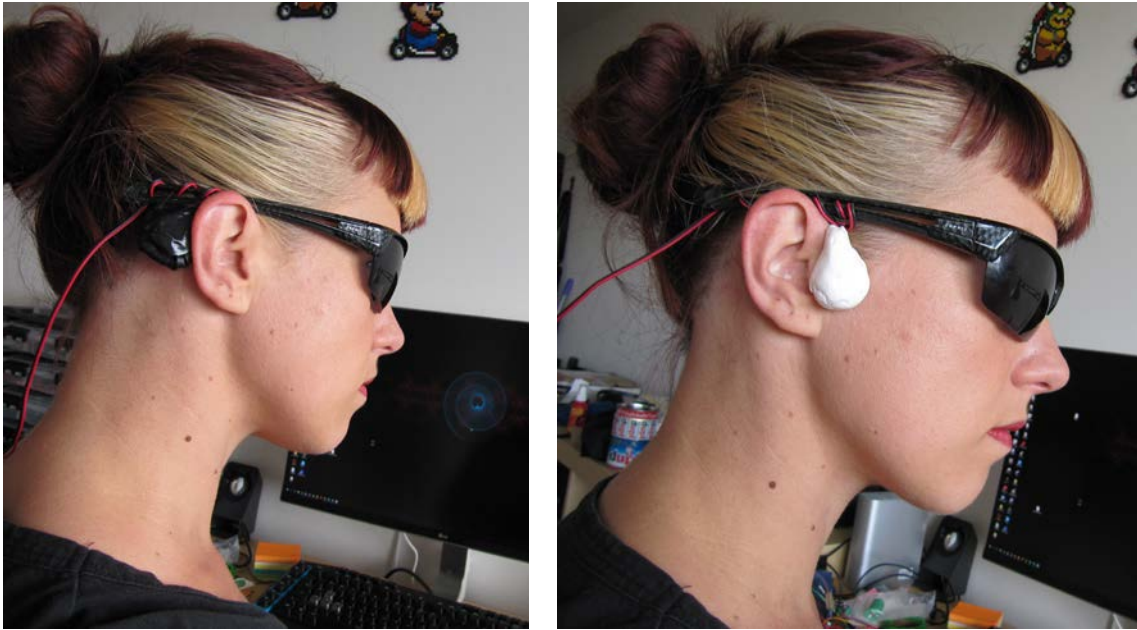
Figure 21: Protosketches exploring cover materials and position of speakers when mounted on sunglasses
