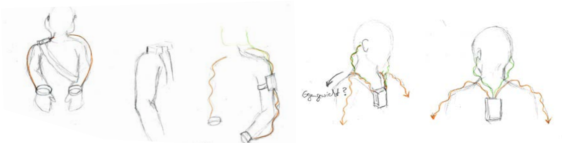
Figure 24: Sketches to explore where on the body to mount the control unit
